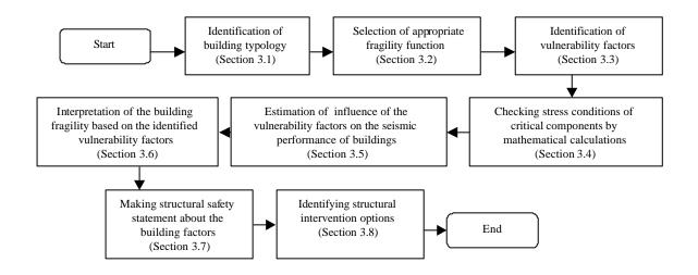
Figure 1: Flow Chart for Structural Vulnerability Assessment
