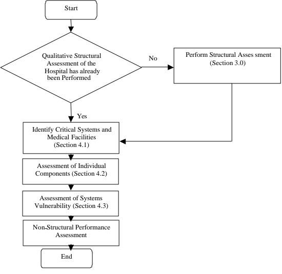
Figure 3: Flowchart for Non-structural Vulnerability Assessment
