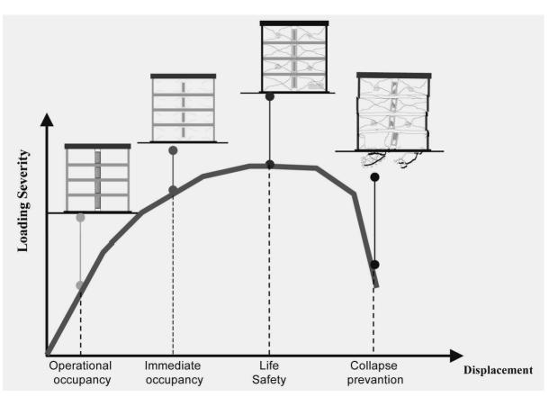
Figure A-XI. 1: Illustration of Building Performance Levels
