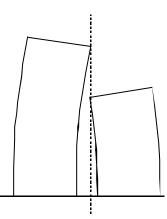
Figure A IV-4: Sufficient gap between two buildings prevents pounding
