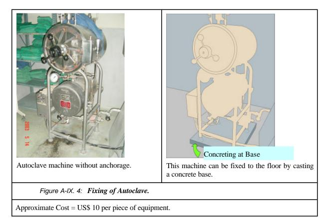
Some equipment and components of a system can easily be bolted to the floor. Transformers, water treatment tanks, communication equipment and control panels of X-ray units are typical examples of equipment that can be anchored to the floor.
