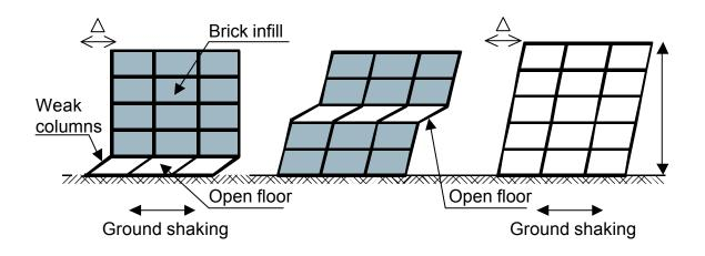
Figure A IV-6: Soft storey due to lack of brick infill
