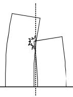
Figure A IV-3: Pounding due to small gap between two buildings
